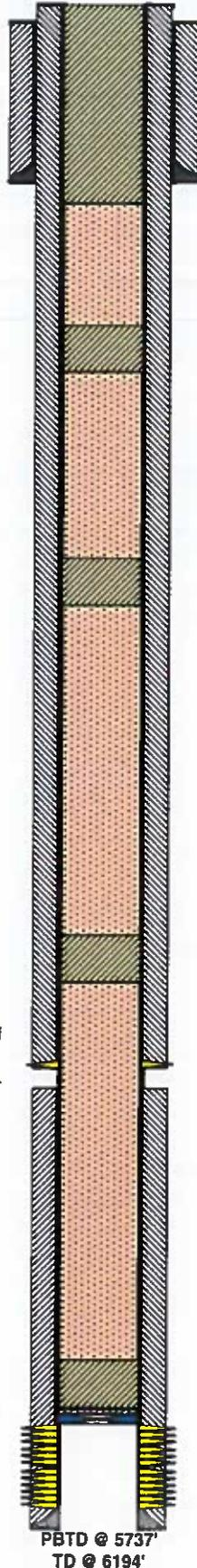
5. PUH & perf @ 557' & attempt to CIRC/sqz 150 sx Class "C" cmt from 557' to surf. (Surf Shoe, Yates, Water Board, & Surf Plug)
