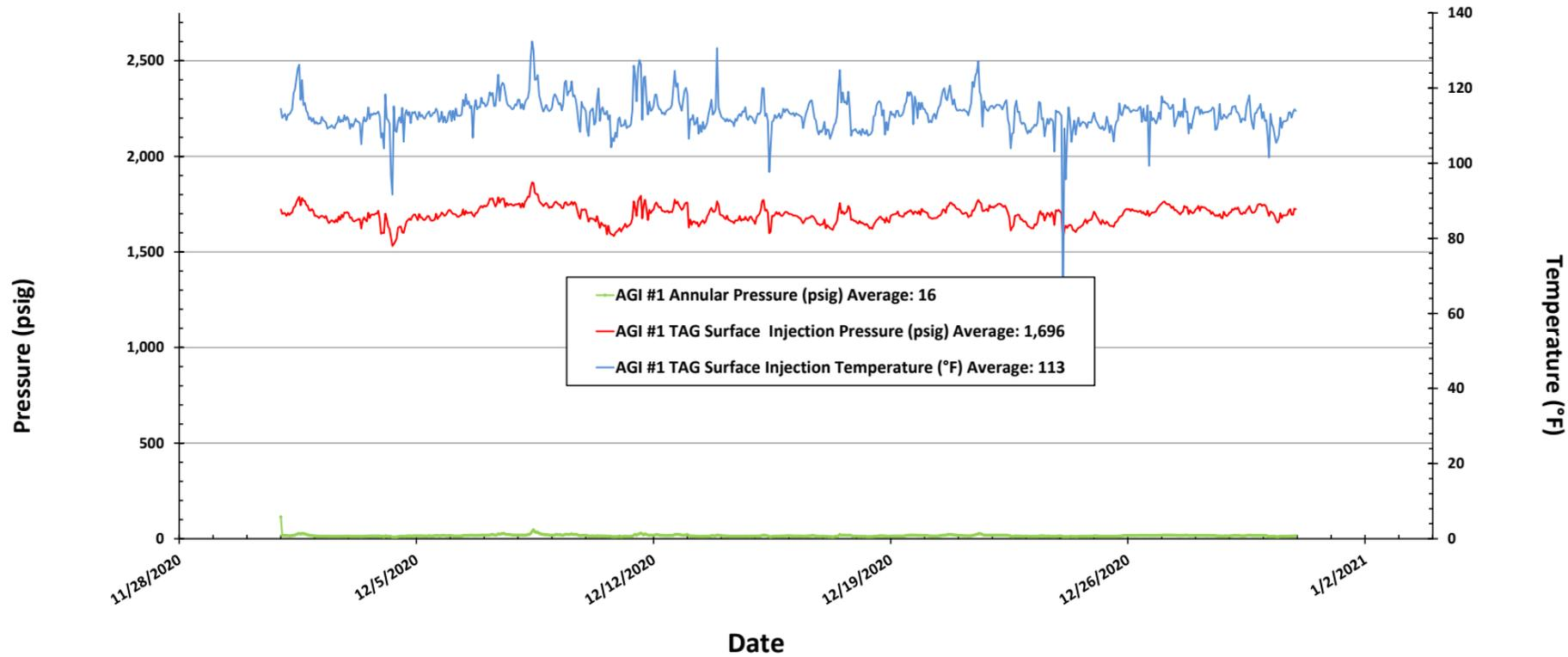
**Figure #4: Linam AGI #1 TAG Injection Pressure and Casing Annular Pressure Differential (psig)**
