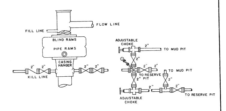
FOR SERVICE 2 M, SCREWED CONNECTIONS MAY BE USED INSTEAD OF FLANGED CONNECTIONS.
