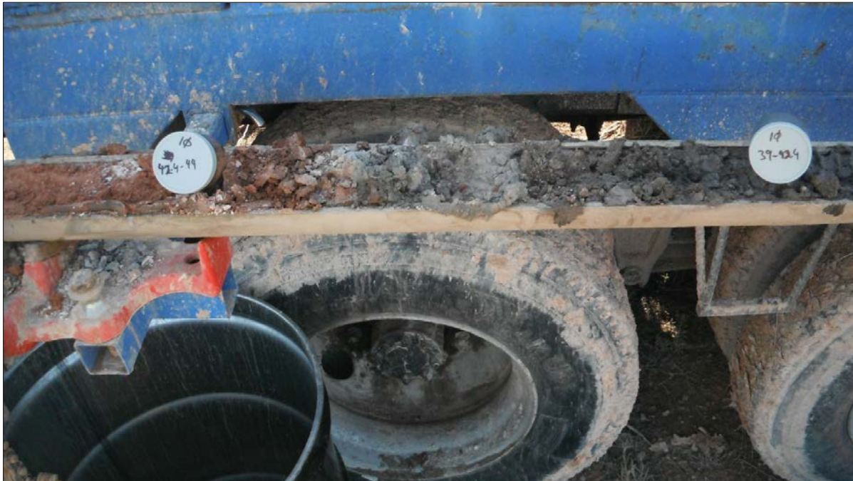
No. 9 – Gray stained sandy soil above red-brown clay in MW-10. Lithologic contact is at about 43 feet bgs.
