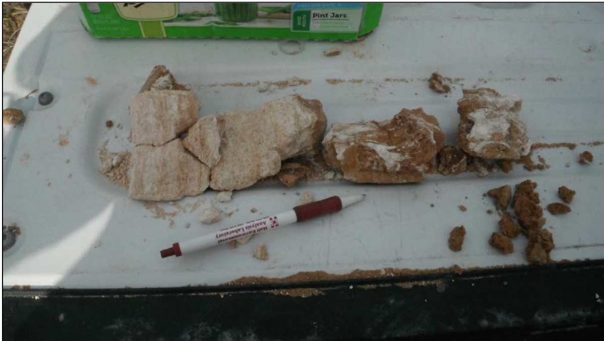
No. 7 – Laminations of caliche in clay underlain by caliche in MW-09.
