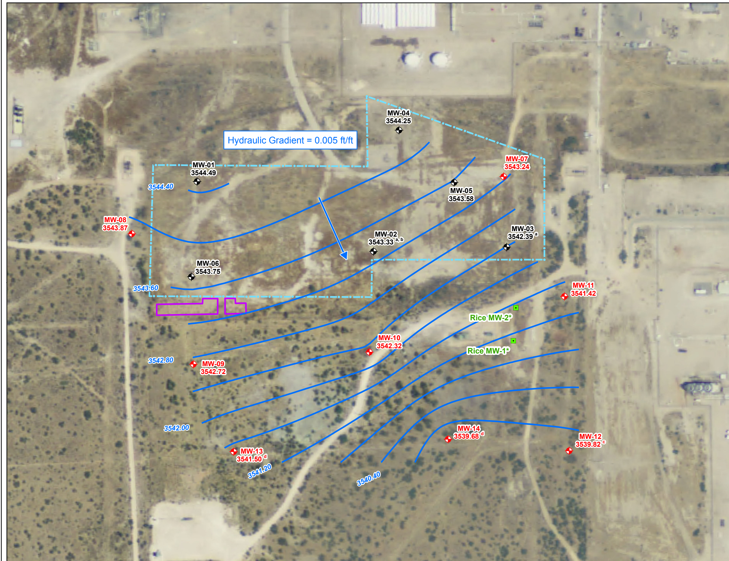
Figure 3 Groundwater Elevations May 22, 2012 Former Enersource Facility Monument, NM
