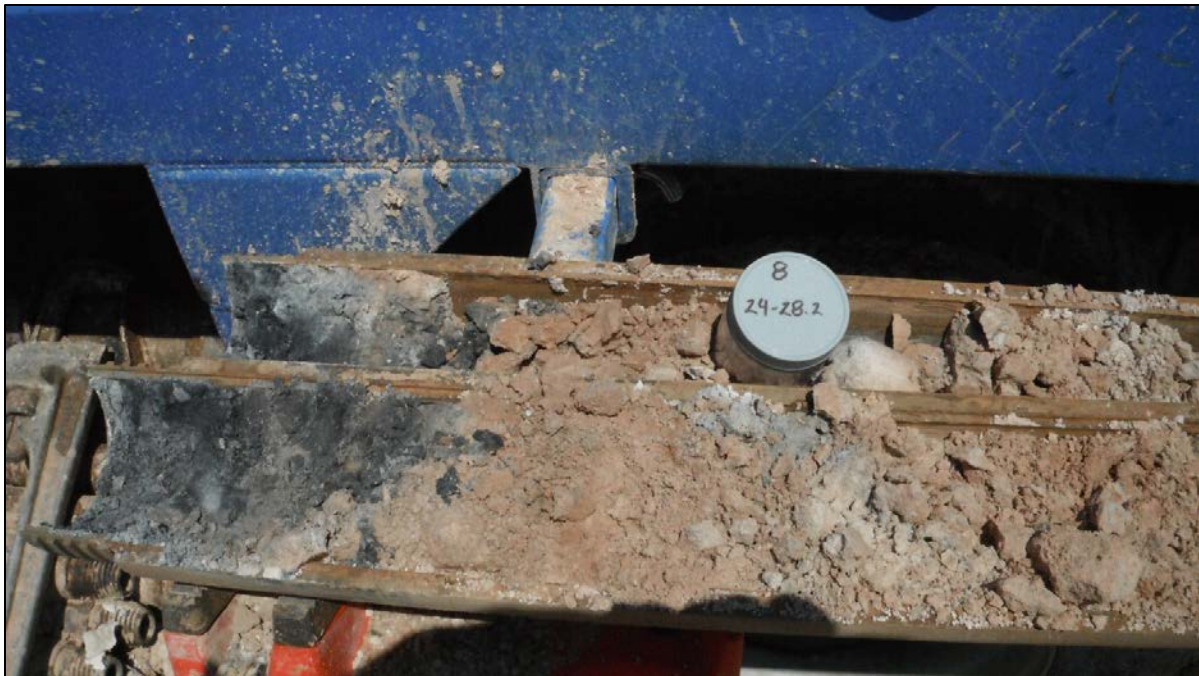
No. 6 – Gray, hydrocarbon staining in MW-08 beginning at approximately 28 feet bgs.
