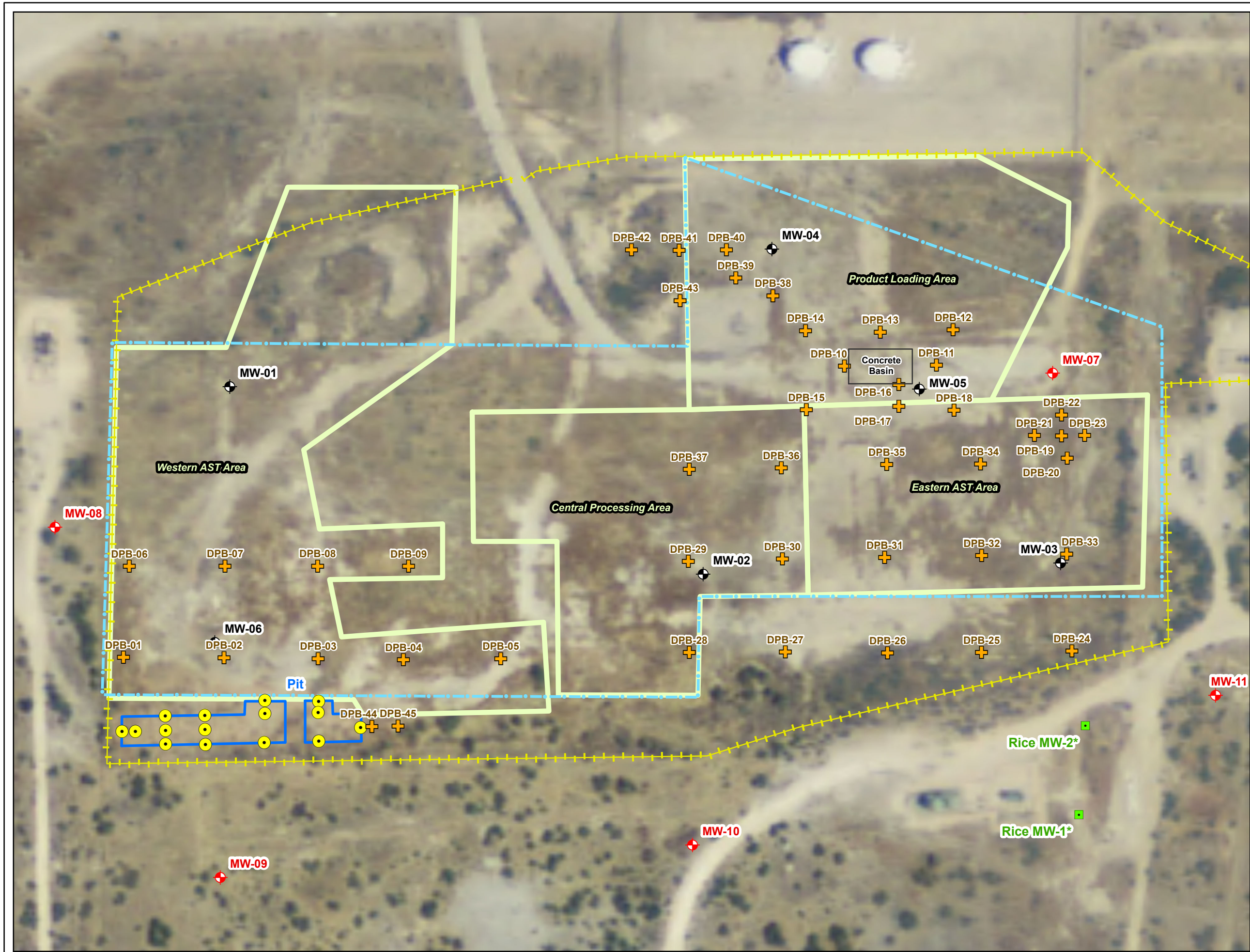
Figure 2b 2009 Soil Boring and Confirmation Sample Locations Former Enersource Facility Monument, NM
