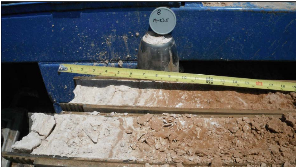
No. 5 – Sand/Caliche contact in MW-08 in core collected from 19 to 23.5 feet bgs.
