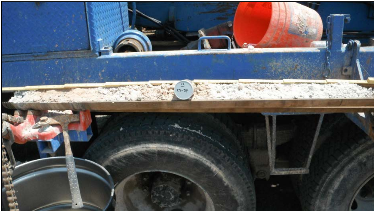
No. 11 – Sand with clay in MW-13 from 29 to 34 feet bgs.
