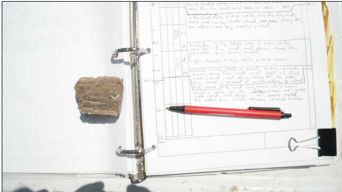
No. 8 – Caliche laminations in silty sand from a depth of approximately 15 feet bgs in MW-10.
