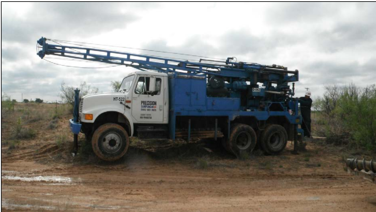
No. 4 – CME 85 setting up to drill MW-08.
