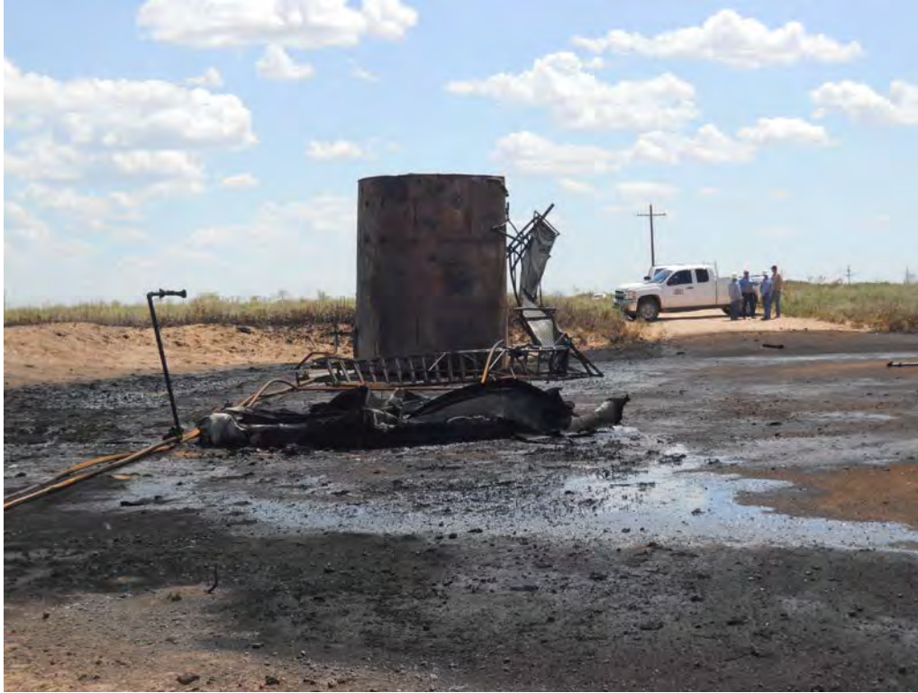
Figure 1 – The remains of the fiberglass produced water tank is in the foreground. One of the two oil tanks is in the background. Some liquid crude is on the location and some of the black material in the photograph is ash from the fire.
