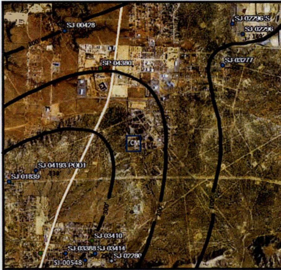
Figure 1: Estimated Depth to Water in Unconfined Aquifer(s)
