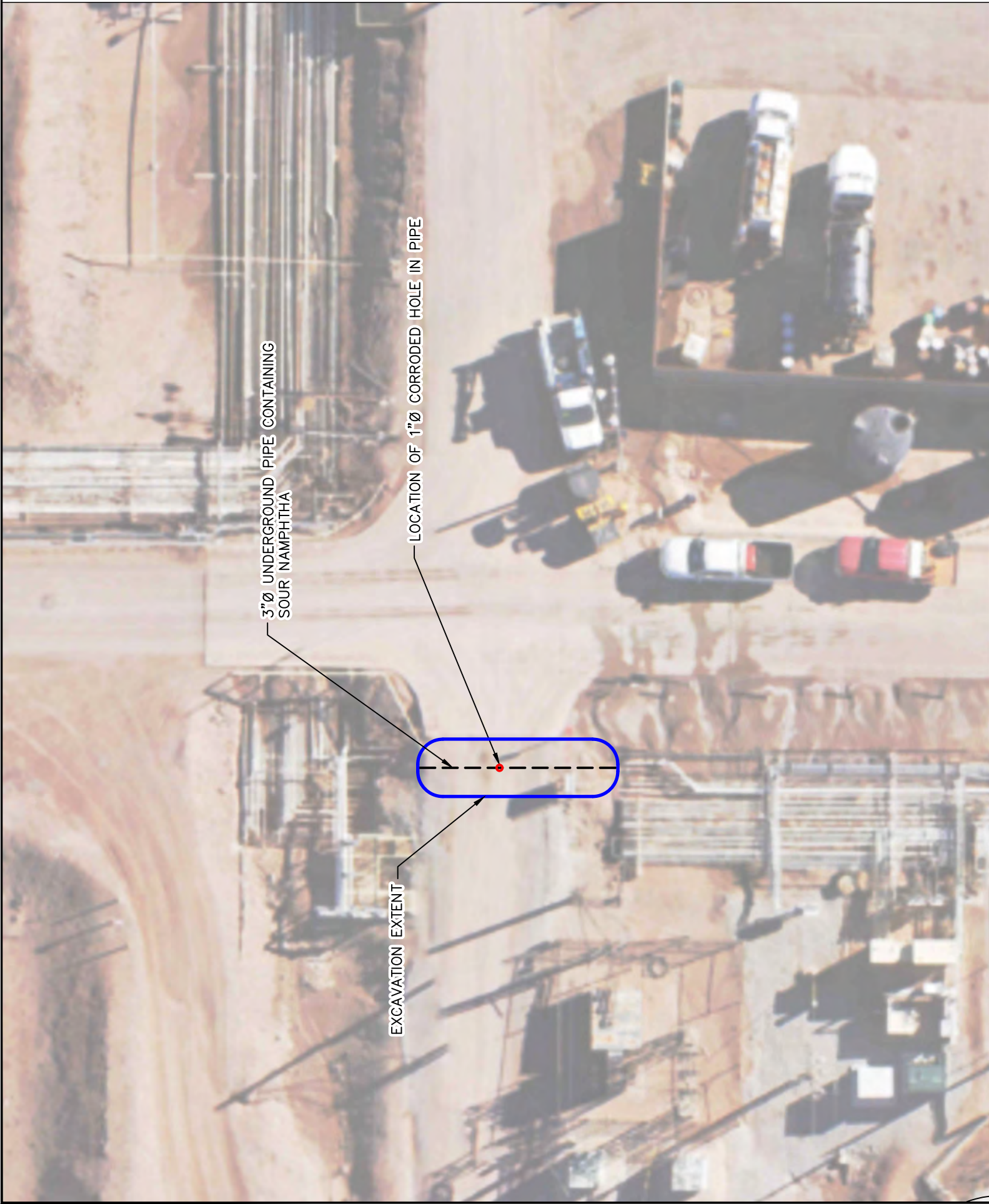
2 SOUR NAPHTHA RELEASE EXCAVATION EXTENT SCALE: 1" = 20'
