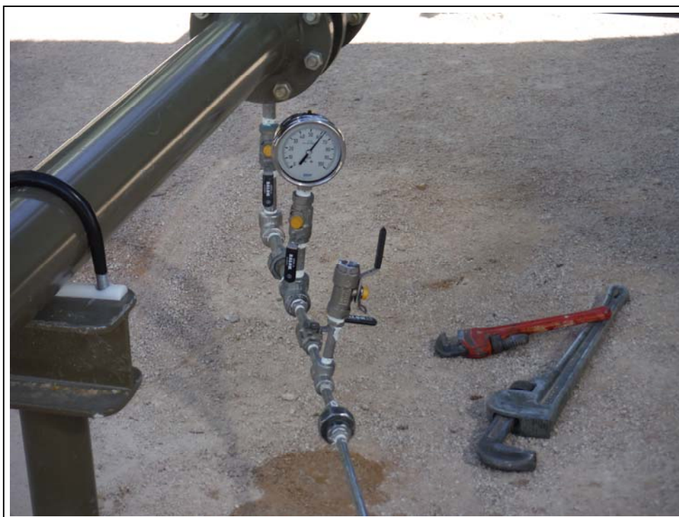
52. Pressure testing of seals and valves at 60 psi.
