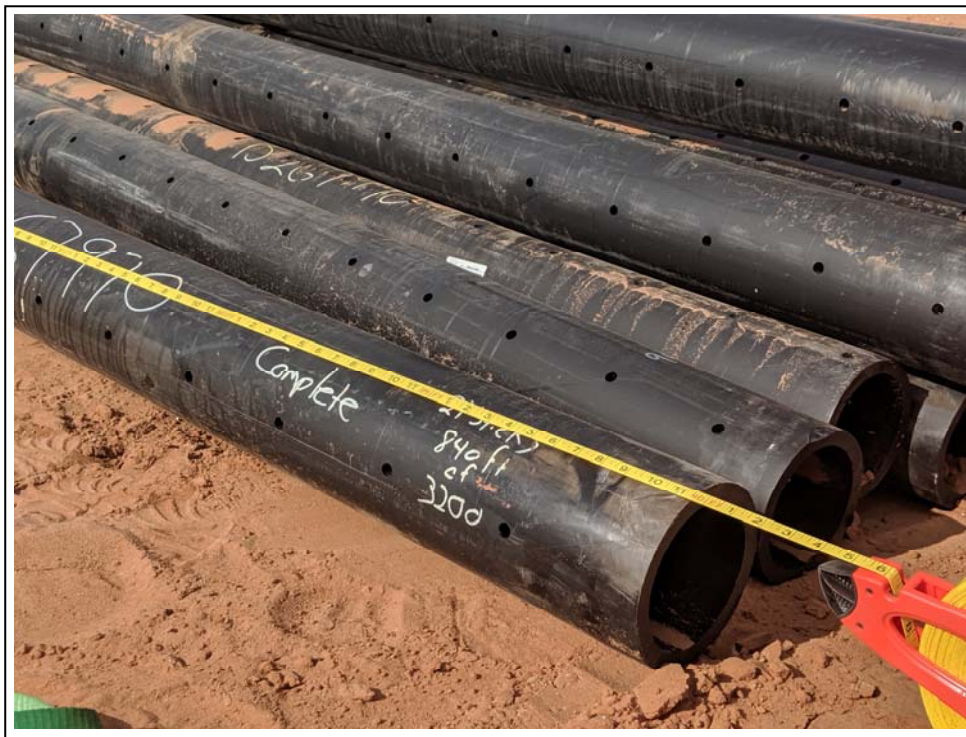
18. 5/29/2019: 6-inch perforated SDR 11 HDPE pipe, 40 feet
