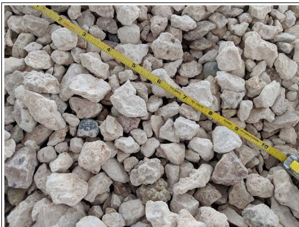
22. 8/22/2019: Select aggregate for leachate collection system
