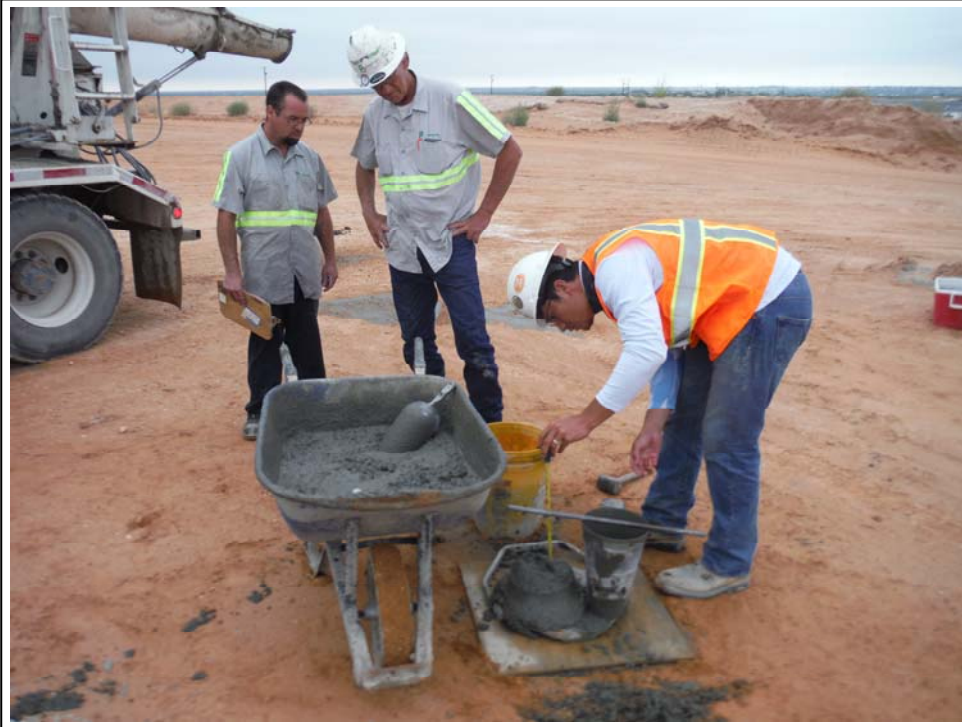
43. 8/28/2019: Beyond Engineering performing a slump test on concrete (view to southwest)
