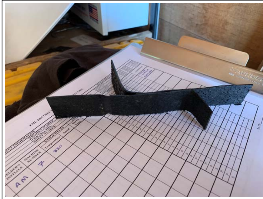
11. 5/20/2019: Pre-weld shear test
