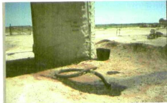
Photo 23 Hose draining oil onto the ground
