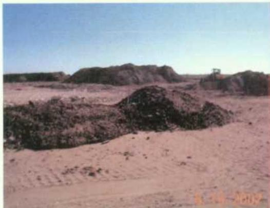
Sludge from heater treaters. Norm contamination. Samples taken and removed from mass of pile show only background.
