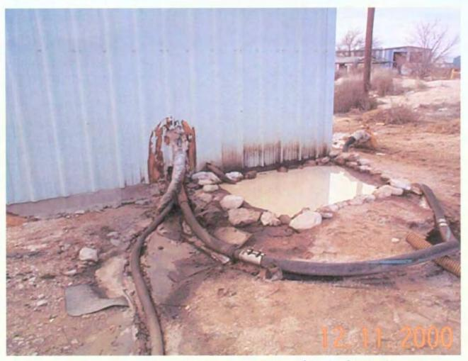
KEY BW-018 WASTE LUBE OIL & WATER POND OVER FLOWING - POND HAS LINER
