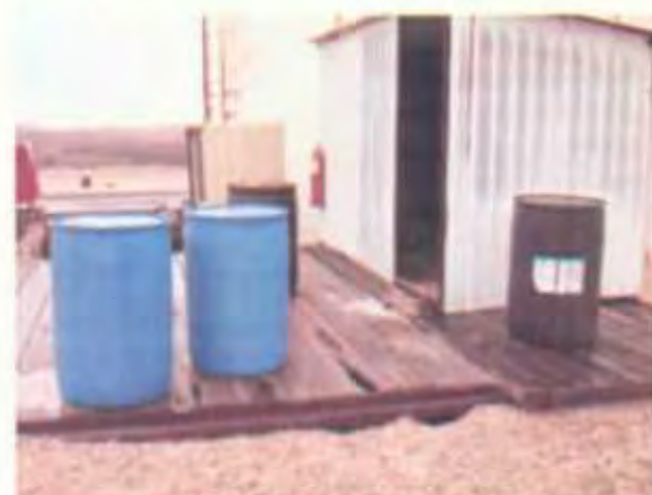
Improper secondary containment and drum storage area
