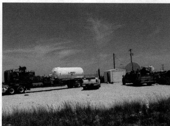
BJ Services N2 truck in position had pumped for 3 minutes to pressure up to 300 psig when I arrived
