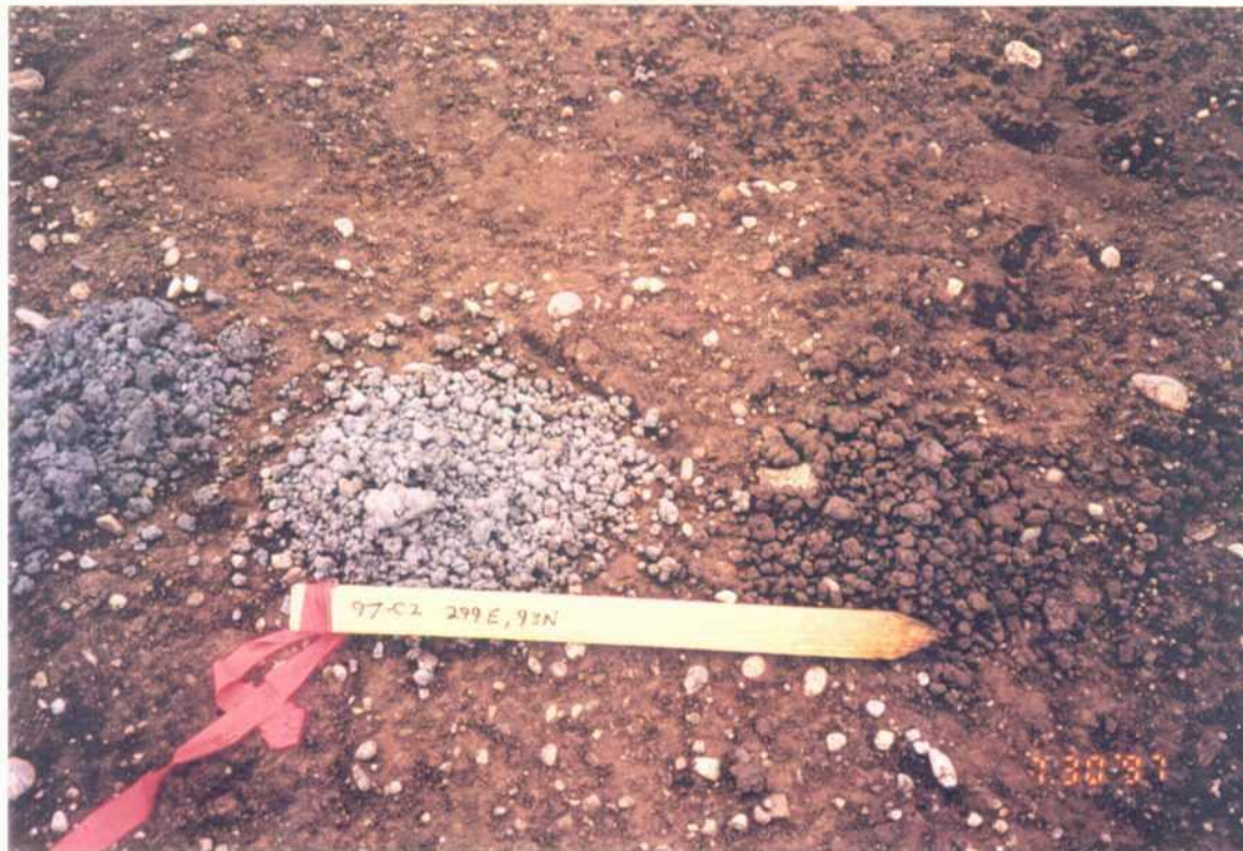
Photograph A-34: Boring 97-C2, left, 9-13 ft.; center, 7-9 ft.; right, 5-7 ft.
