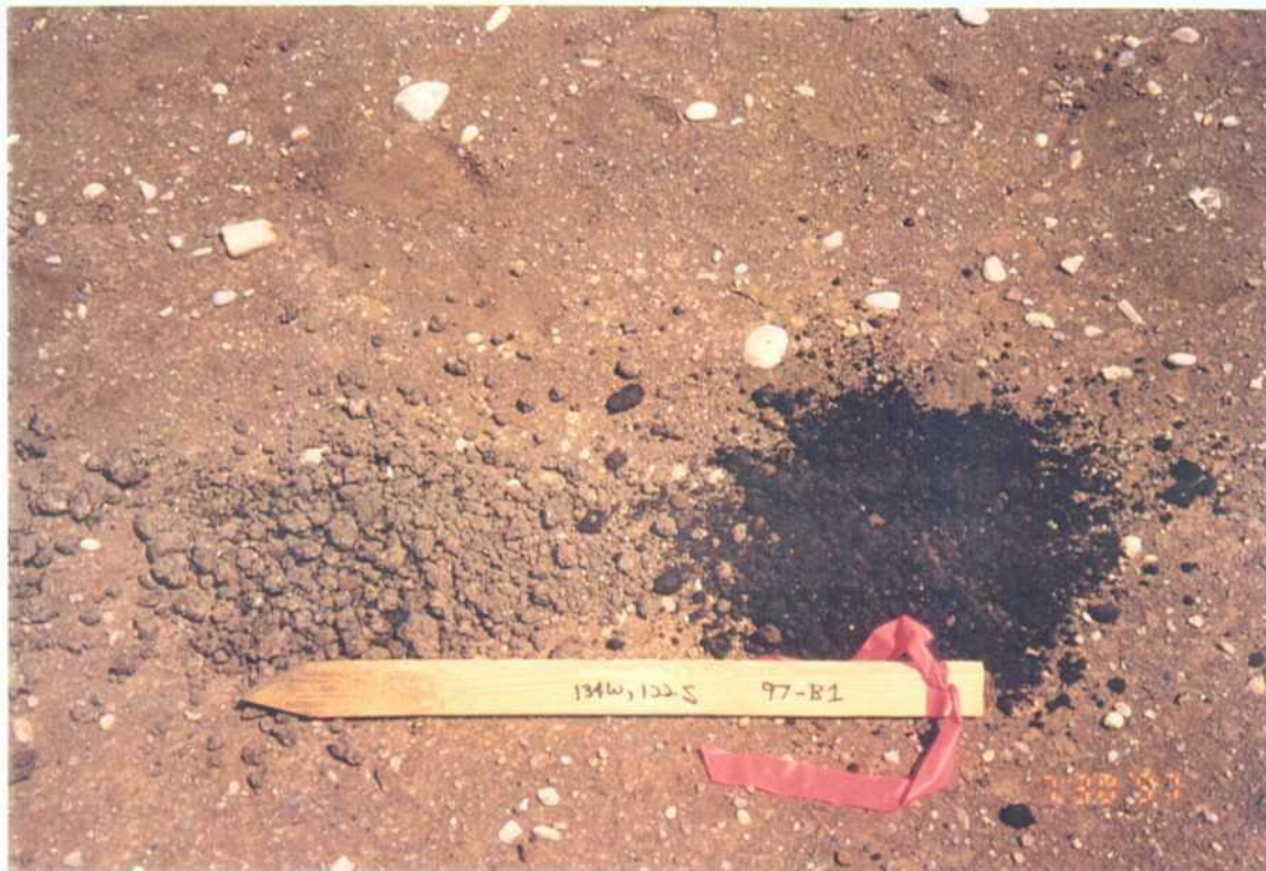
Photograph A-17: Boring 97-B1, left 2-5 ft.; right 0-1 ft.
