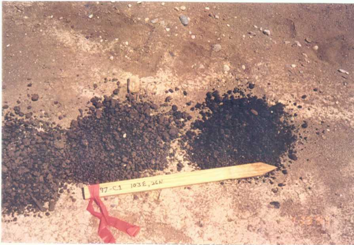
Photograph A-29: Boring 97-C1, left, 5-8 ft.; center, 2-5 ft.; right, 0-2 ft.
