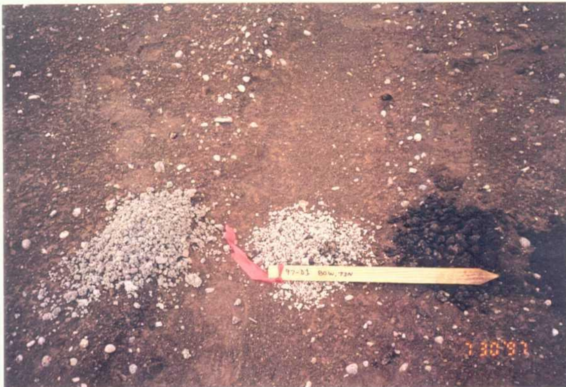
Photograph A-38: Boring 97-D1, left, 12-15 ft.; center, 10-12 ft.; right, 7-10 ft.
