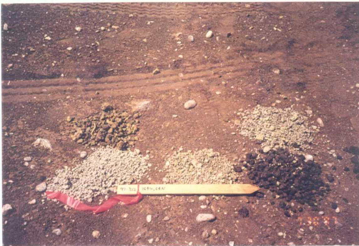
Photograph A-42: Boring 97-D2, left top, 14-15.5 ft.; left bottom, 12-14 ft.; center, 10-12 ft.; right top, 9-10 ft.; right bottom, 7-8 ft.
