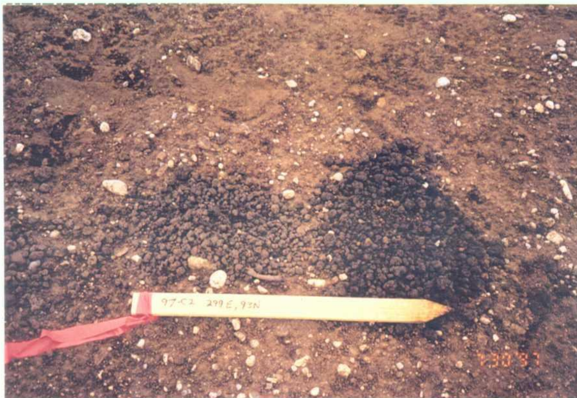
Photograph A-33: Boring 97-C2, left, 2-5 ft.; right, 0-2ft.
