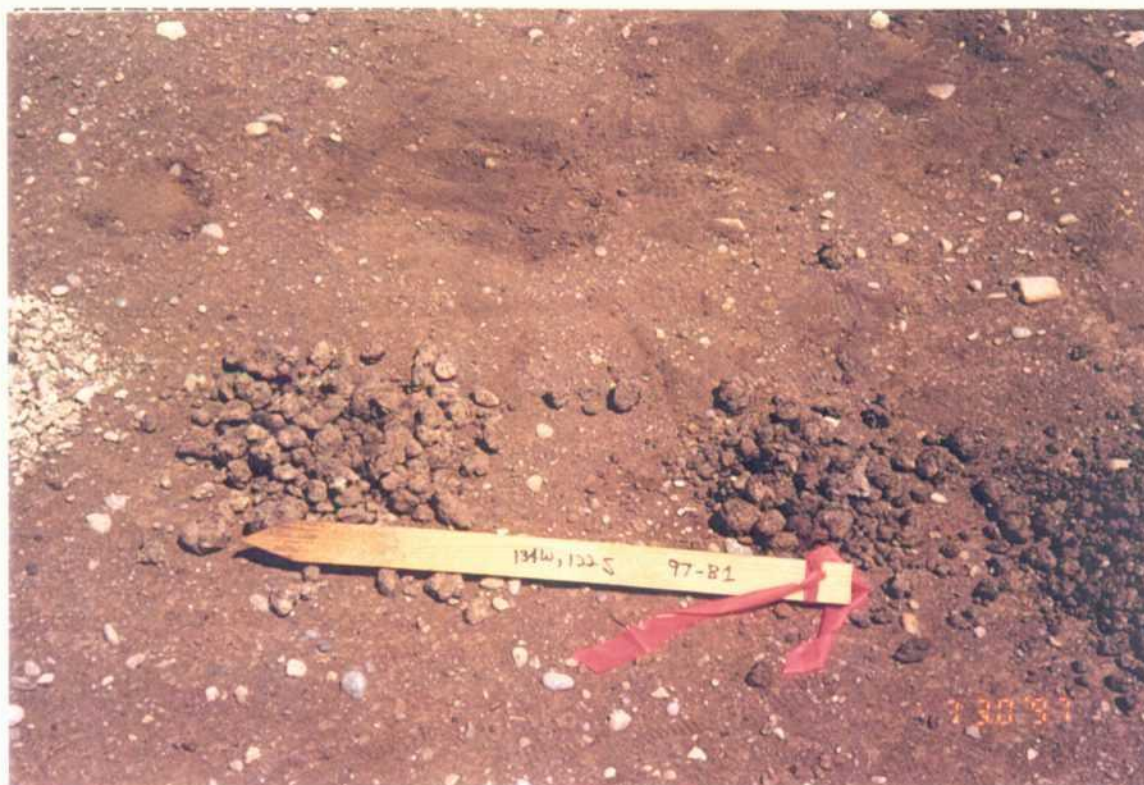
Photograph A-18: Boring 97-B1, left 8-10 ft.; right 5-8 ft.
