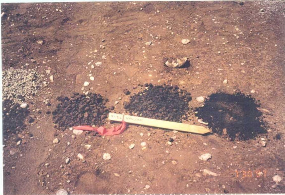
Photograph A-41: Boring 97-D2, left, 5-7 ft.; center, 2-5 ft.; right, 0-2 ft.
