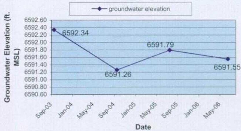
WMW-6 Groundwater Elevation Graph
