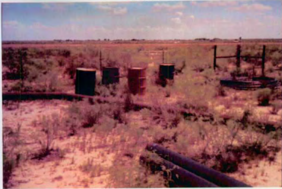
GW-141 CROSSTEX ENERGY SERVICES LOVING GAS PLANT Unlabeled drums and other containers improperly stored
