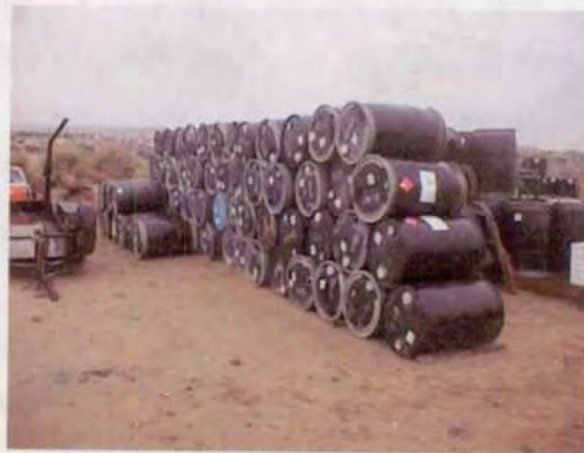
Pic6- Empty drum storage area. No containment and bungs were not aligned horizontally.
