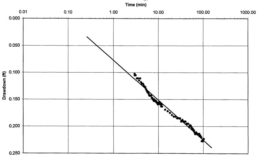
MW-4 7.0 gpm
