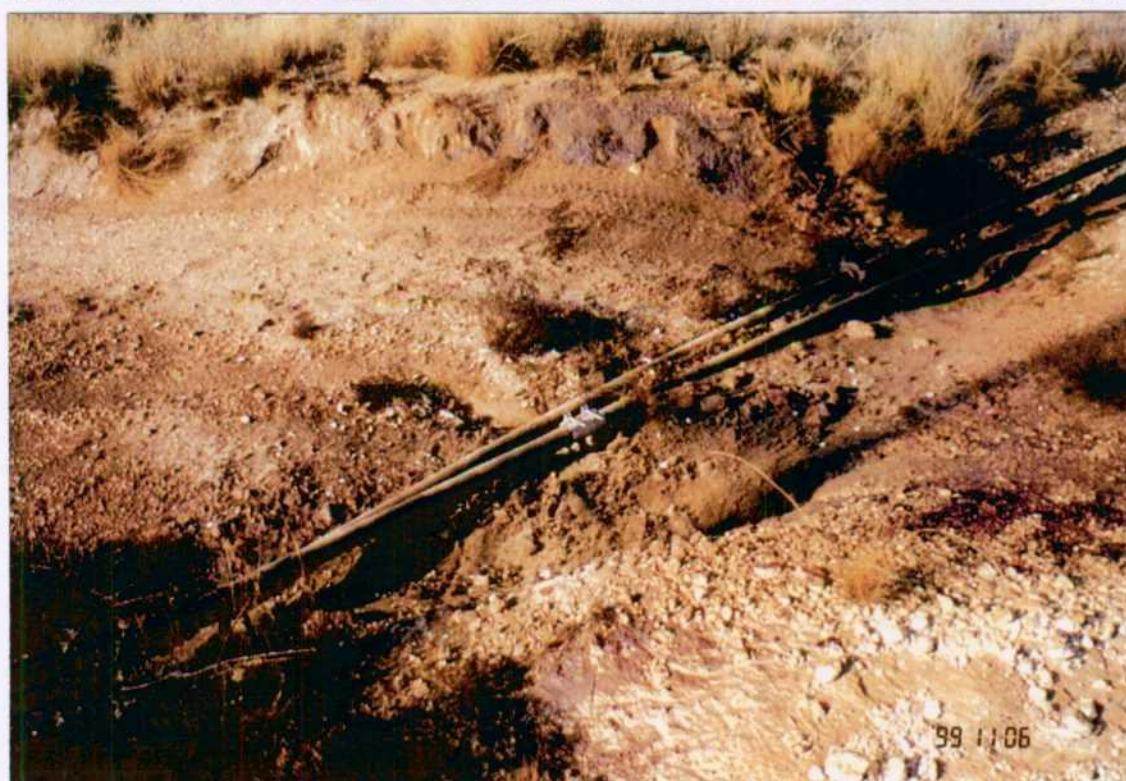
MARALO TALMAT YATES UNIT. 11-6-99 Flow Line LEAK FROM Well #22
