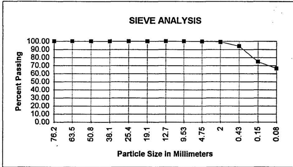
**Soil Classification (USCS):** *Sandy Lean Clay to Silty Clay (CL): Grey brown to medium yellow orange, slightly plastic, with fine to very fine sand. Larger sand particles consisted of calcified fine sand clusters.*
