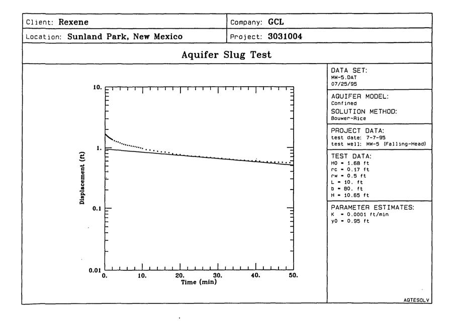
Client: Rexene Company: GCL Location: Sunland Park, New Mexico Project: 3031004 Aquifer Slug Test DATA SET: MW-6S.DAT 07/25/95 AQUIFER MODEL: Confined SOLUTION METHOD: Bouwer-Rice PROJECT DATA: test date: 7-6-95 test well: MW-6S (Falling-Head) TEST DATA: HO = 1.78 ft rc = 0.17 ftrw = 0.5 ft L = 10. ft b = 80. ft H = 11.89 ftPARAMETER ESTIMATES: 0.1 K = 0.0009 ft/miny0 = 1.4 ft0.01 10. 40. 50. 30. Time (min) AQTESOLV
