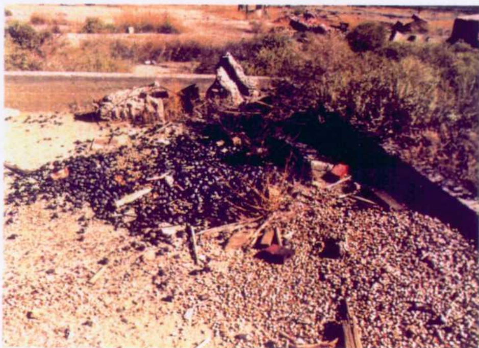
Photo 10. Lewis 890627 Rashig rings used in tower packing located in the base of a building foundation.
