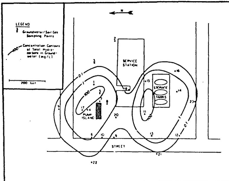
Figure 3: Distribution of total hydrocarbons in shallow groundwater underlying a gasoline service station.
