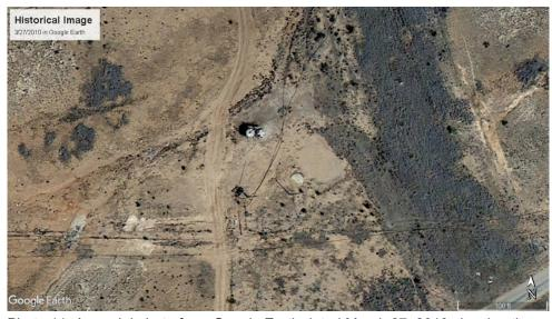
Photo 11. An aerial photo from Google Earth dated March 27, 2010 showing the small pumping unit that remains approximately 60 feet south-southwest of sampling location SS-5 and two above-ground storage tanks whose previous locations were approximately 25 feet north of SS-5. Note stained soil in the vicinity of the two tanks.
