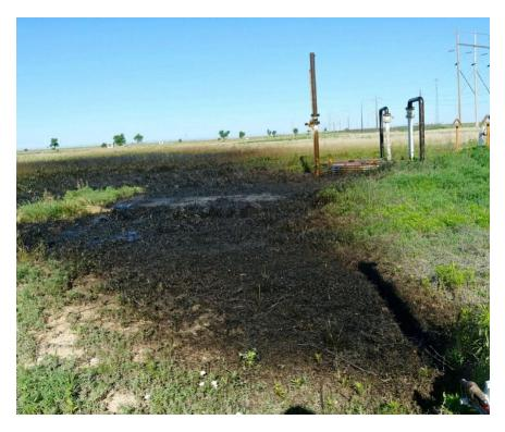
FIG. 8- FIVE (5) HOURS POST-TREATMENT FIELD SERVICE MIDSTREAM CLIENT OKLAHOMA. HYDROCARBON RELEASE ON SOIL AND VEGATATION. (R3ICS, LLC. 2019 JUNE)
