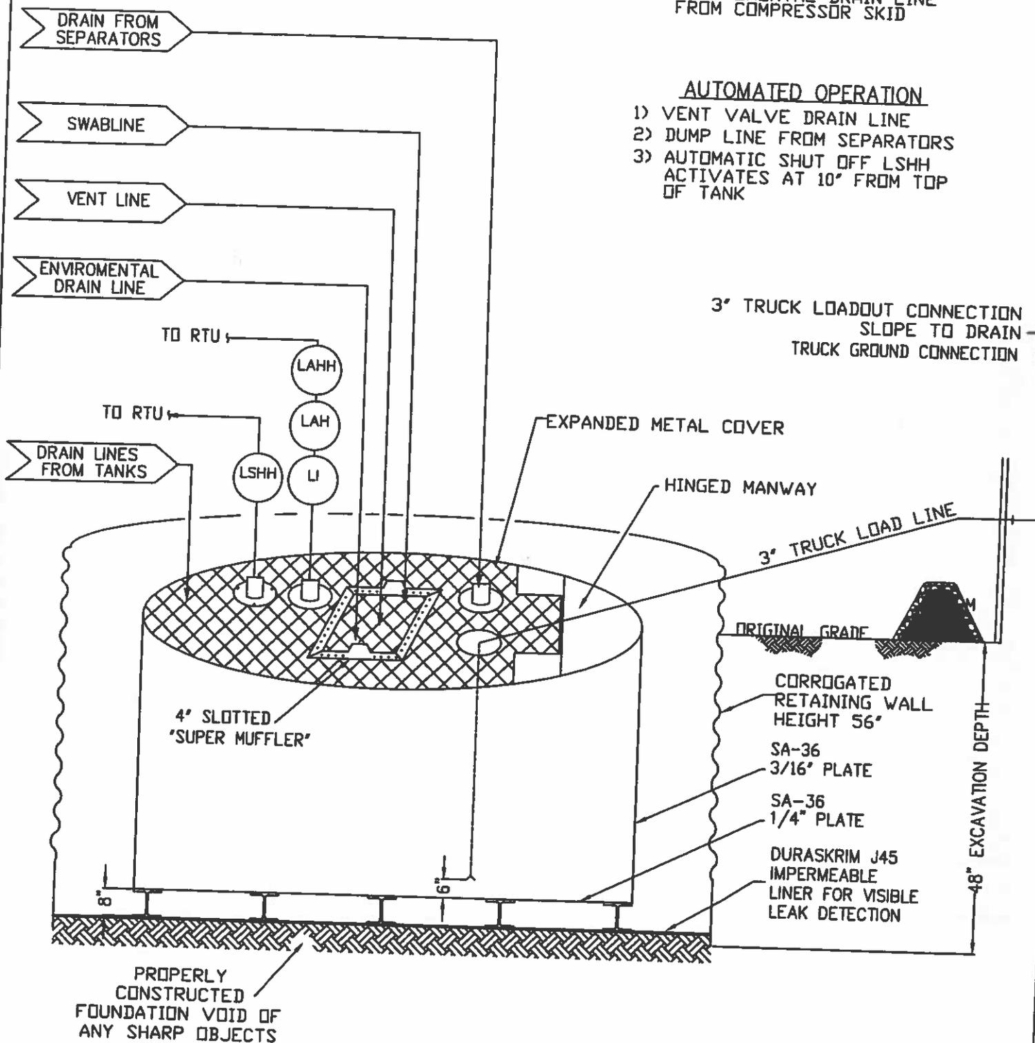
3" TRUCK LOADOUT CONNECTION
