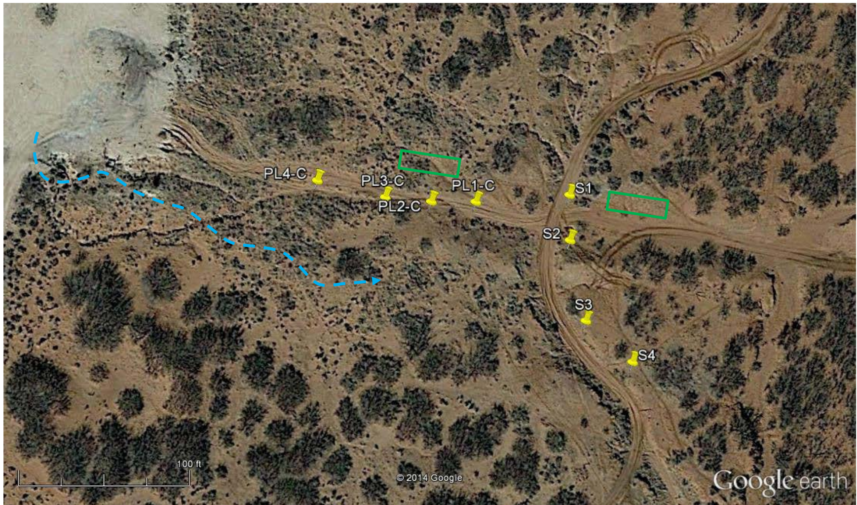
Plate 1: Google Earth image showing sample locations and drainage pattern to be re-established (dashed blue line). The original drainage is visible in the 10/21/96 Google Earth image. The green rectangles are the locations of the east (right) and west (stockpile).
