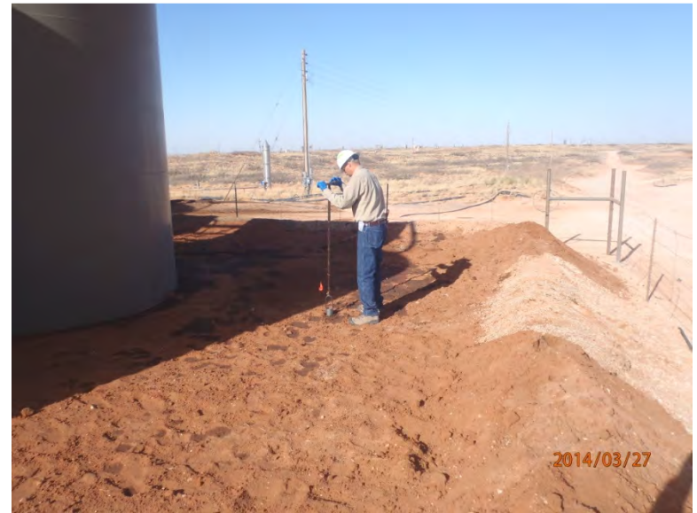
Hand augering for depth, facing west 3/27/14
