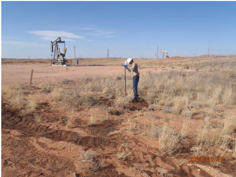
Hand augering for depth, facing southwest 3/27/14
