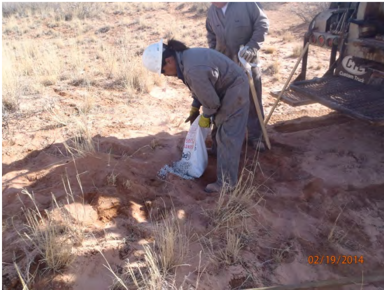
Plugging SB-1 in total with bentonite 2/19/14
