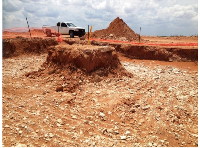
SP-12. Sample from approximate center of excavation, scrapings from bottom in hard caliche. Right photo looking southwest from approximate center of excavation.
