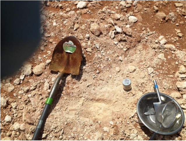
SP-12. Sample from approximate center of excavation, scrapings from bottom in hard caliche. Right photo looking southwest from approximate center of excavation.
