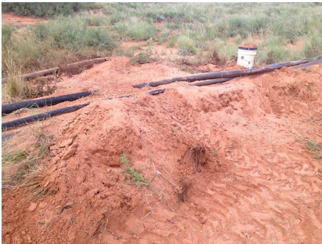
Release Point #2 – Damage caused by dozer treads – only location of product release from damage line.
