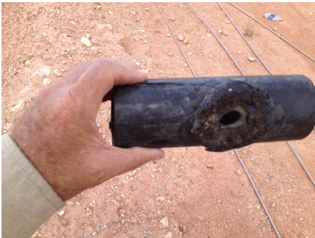
Leak #1 - Flowline section damaged by vehicle exhaust
