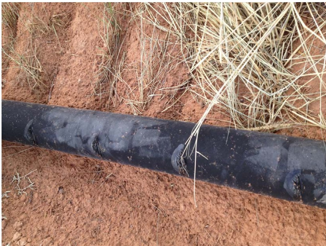
Leak 2 – Damage caused by bulldozer – NOTE: no product release at this damage site
