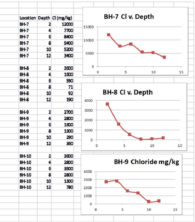
The data allow me to predict that we will see near background chloride levels about 20 feet below grade at this deep boring
