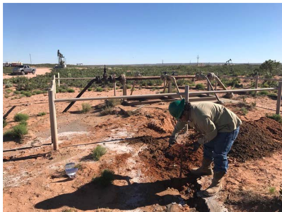
Collecting sample by hand auger
