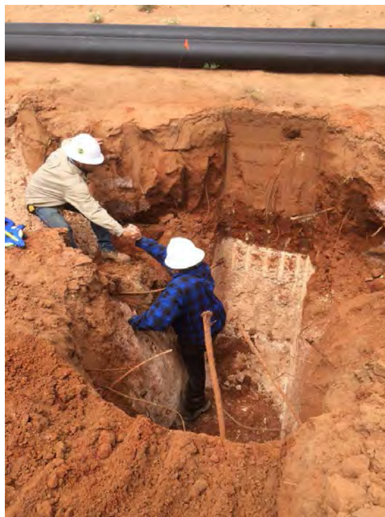
Figure 2: Sampling trench Pooling-02 with a total depth of 9-feet below ground surface. A silty sand composes the upper 4.5-feet. Below 4.5-feet white caliche is visible at the lower depths of the sampling trench. GPS: 32.4451056 N, -103.6040639W. Date/time: 2019-08-03 11:29:24
