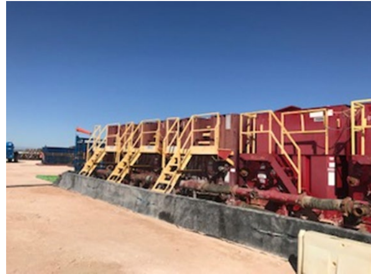
Photograph 2: Southeast view of frac tanks with secondary lined containment.
