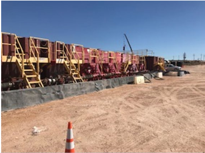
Photograph 1: Northeast view of frac tanks with secondary lined containment.
