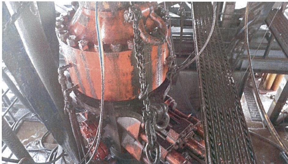
Figure 1: Winch System attached to BOP Stack
