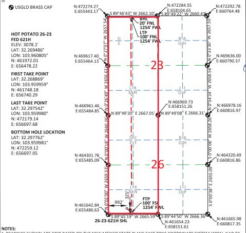
1. BEARINGS SHOWN ARE GRID BASED ON THE NEW MEXICO STATE PLANE EAST ZONE COORDINATE SYSTEM (3001), NAD 83 (2011), BASED FROM GPS OBSERVATIONS, OCCUPYING A WHS CONTROL POINT (5/8" REBAR), LOCATED AT NORTH: 456034.443, EAST: 653560.641, ELEVATION: 3101.4, DETERMINED BY AN OPUS SOLUTION ON MOVEMBER 9TH, 2019. 2. DISTANCES DEPICTED HEREON ARE REPORTED AS GROUND DISTANCE IN US SURVEY FEET USING A COMBINED SCALE FACTOR OF 1 000220989
