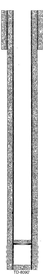
12-1/4" hole @ 1230' 9-5/8" csg @ 1230' w/ 800sx-TOC-Surf-Circ
