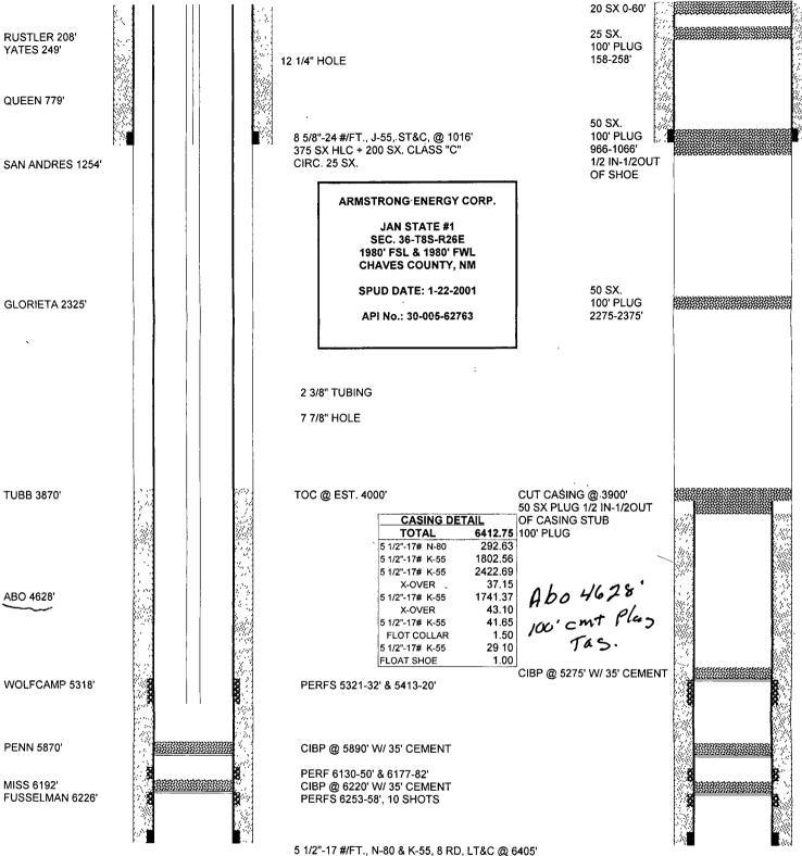
5 1/2 - 17 #/F1., N-80 & K-55, 8 RD, LT&C @ 6405' 400 SX 35/65 POZMIX W/ 2% GEL,, .3% HALAD-4, .2% CFR-2, 5 #/SX SALT TOC @ EST. 4000'
