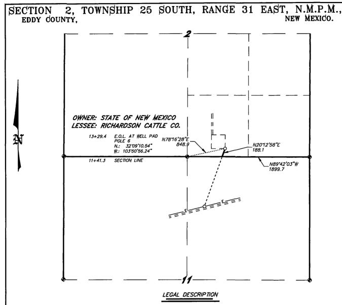
A STRIP OF LAND 30.0 FEET WIDE, LOCATED IN SECTION 2, TOWNSHIP 25 SOUTH, RANGE 31 EAST, N.M.P.M., EDDY COUNTY, NEW MEXICO AND BEING 15.0 FEET LEFT AND RIGHT OF THE FOLLOWING DESCRIBED CENTERLINE SURVEY.
