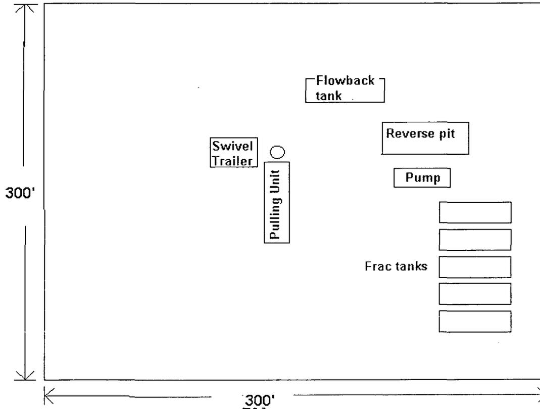
Note: Flowback tank is a frac tank, Reverse pit is a steel open top tank measuring 20' L x 7' W x 6' D.
