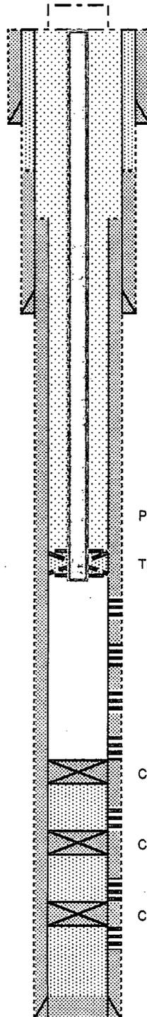
Well head - Welded on 9 5/8" extension @ re-entry.
