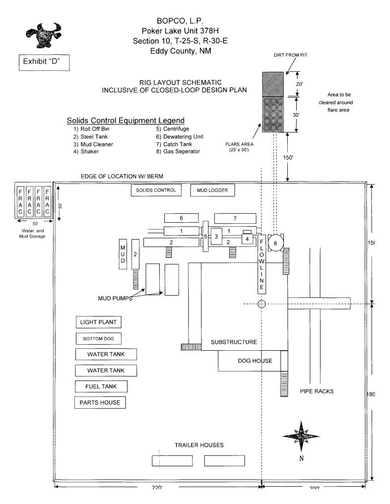
Wtd-ser/Drilling/DrillingDiagrams/H&P Drilling Rig Pad deminsions - Closed LoopRes Pit Exibit D w-rig
