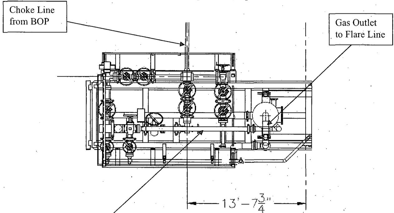
**Choke Manifold – Gas Separator (Side View)**
