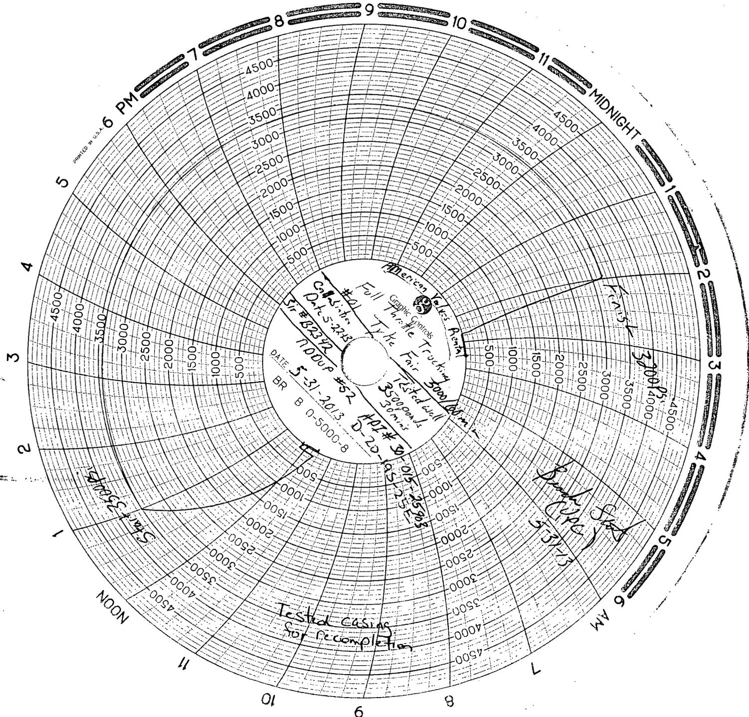
Tested casing for re completion
