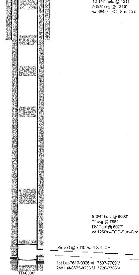
12-1/4" hole @ 1215' 9-5/8" csg @ 1215' w/ 684sx-TOC-Surf-Circ
