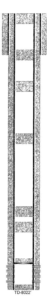
12-1/4" hole @ 1215' 9-5/8" csg @ 1206' w/ 655sx-TOC-Surf-Circ
