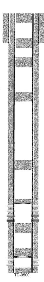
12-1/4" hole @ 1194' 9-5/8" csg @ 1194' w/ 850sx-TOC-Surf-Circ
