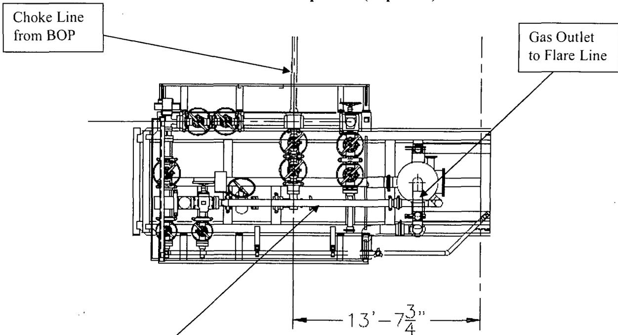
**Choke Manifold – Gas Separator (Side View)**
