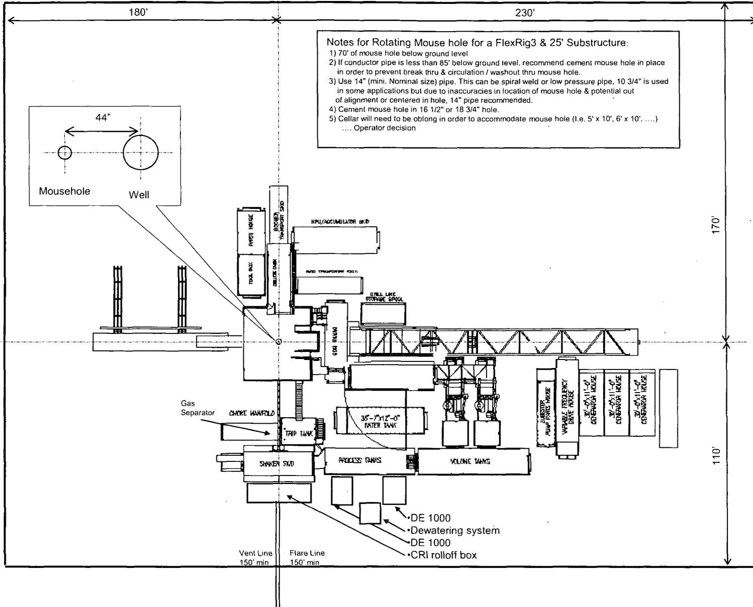
Notes for Rotating Mouse hole for a FlexRig3 & 25' Substructure:
