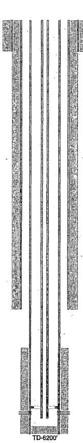
17-1/2" hole @ 504' 13-3/8" csg @ 504' w/ 530sx-TOC-Surf-Circ
