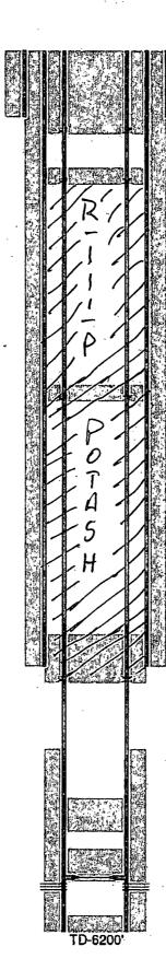
17-1/2" hole @ 504' 13-3/8" csg @ 504' w/ 530sx-TOC-Surf-Circ
