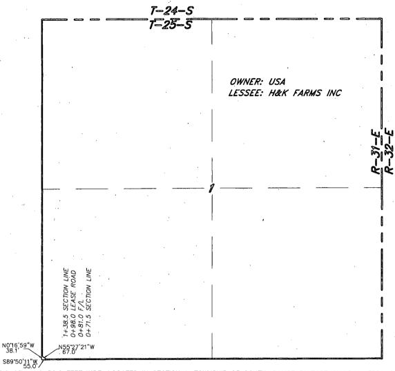
A STRIP OF LAND 30.0 FEET WIDE, LOCATED IN SECTION 1, TOWNSHIP 25 SOUTH, RANGE 31 EAST, N.M.P.M., EDDY COUNTY, NEW MEXICO AND BEING 15.0 FEET LEFT AND RIGHT OF THE ABOVE PLATTED CENTERLINE SURVEY.
